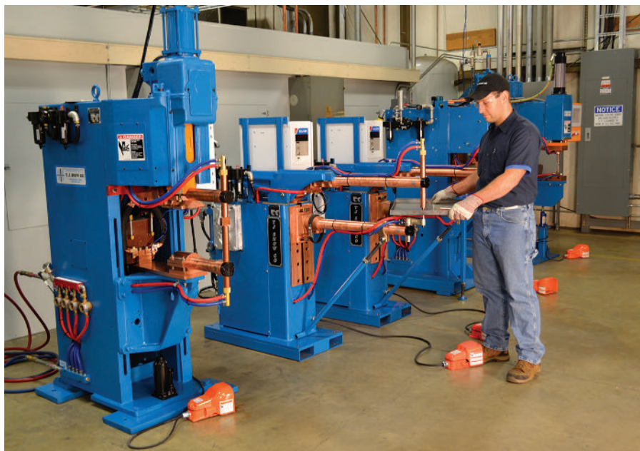
Fig. 1 — If you're looking for the right resistance welding machine for your facility, the rocker arm spot welding machine is less expensive and more versatile.
