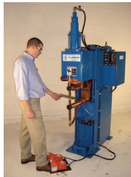
Fig. 2 — The vertical action press-type spot welding machine is recommended when weld appearance needs to be optimized.
