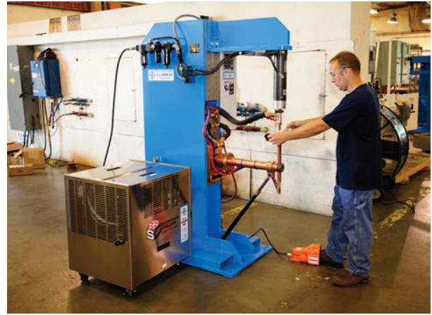
Fig. 3 — Standard spot welding machines, both vertical action and rocker arm types, can be operated safely if an operator holds the parts with both hands outside the pinch point area. Safety can be enhanced by minimizing the opening between the tips and by a control feature called Soft Touch.
