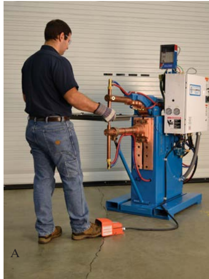
Fig. 2 — A — A rocker-arm spot welding machine with a prominently displayed pinch point warning sign; B — a close-up view of a warning sign.
