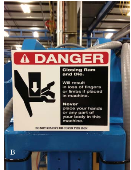
Fig. 2 — A — A rocker-arm spot welding machine with a prominently displayed pinch point warning sign; B — a close-up view of a warning sign.
