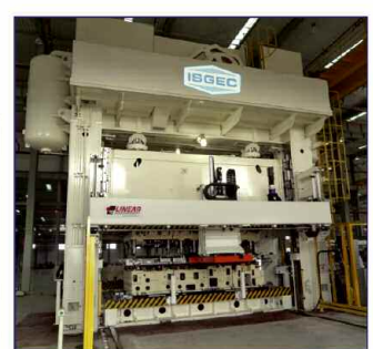
12500 kN Transfer Press supplied to LEAR CORPORATION, USA for China Project (Bolster: 217" x 98" Speed: 15-30 spm, Stroke: 26")
