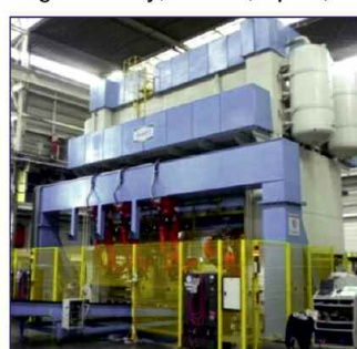
20000 kN Link Drive Transfer Press supplied to BRANDL MASCHINENBAU, Germany with 5 die cushion stations of 640 kN each (Bolster: 240" x 110", Speed: 8-16 spm, Stroke: 39")
