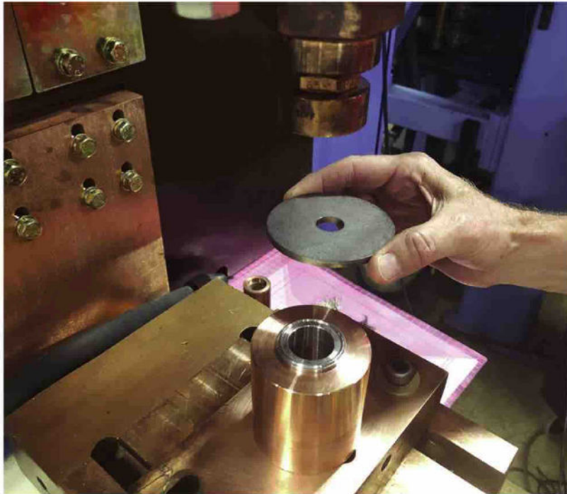
Shown here, an example of typical part geometry and tooling for a part being welded using capacitor-discharge welding. Notice the ring projection.
