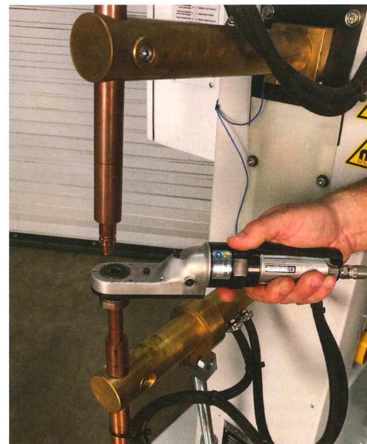
Fig. 2—An operator can use a pneumatic weld-tip-dressing tool while the tips remain installed in the welding machine.
