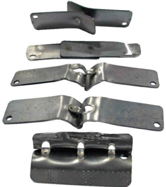
The RSW process looks simple, but fabricators must understand well, and control, the process variables in order to achieve the desired results: a weld stronger than the parent material (illustrated here by a series of pull-test samples).
