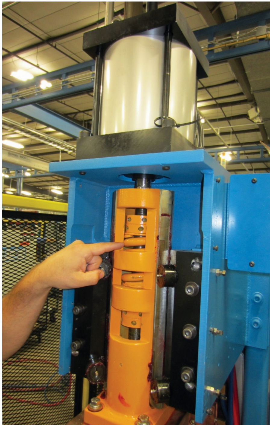
Fig. 1 — Photo of a fast follow-up spring installed in the ram of a projection welding machine.
