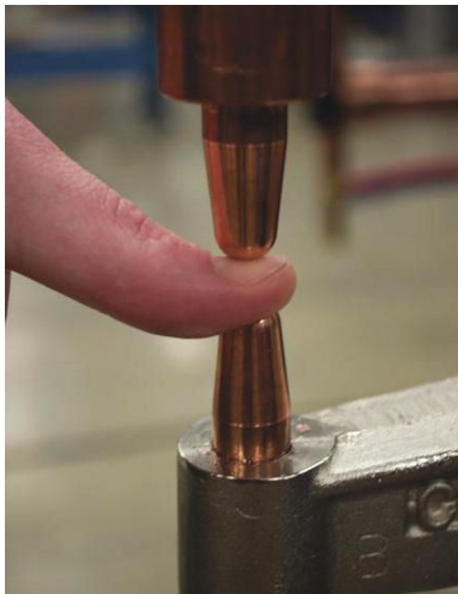
The "pinch point" between the welding tips can be potentially dangerous. Picture courtesy of T.J. Snow Co.
