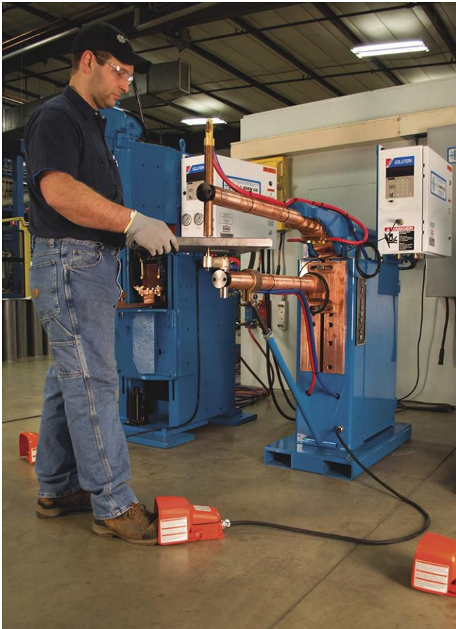
A standard air-operated rocker arm spot welder is very safe to use, but operators should still take precautions. Picture courtesy of T.J. Snow Co.
