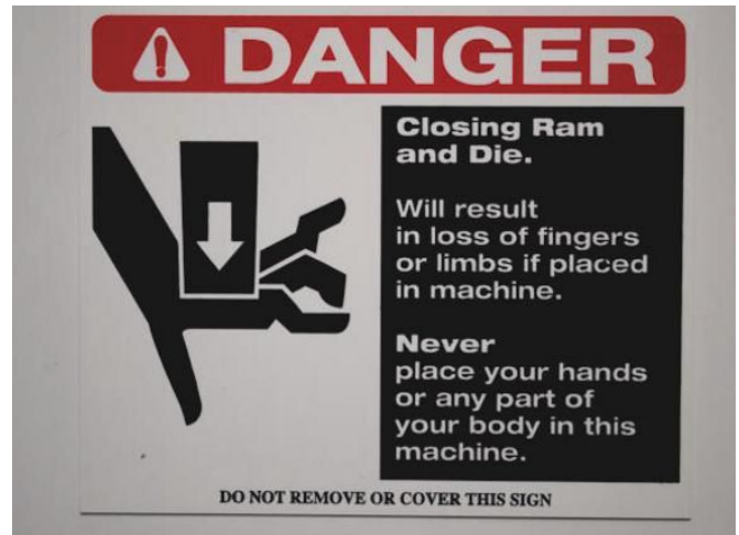
A warning sign similar to this should be on every spot welder. Picture courtesy of T.J. Snow Co.
