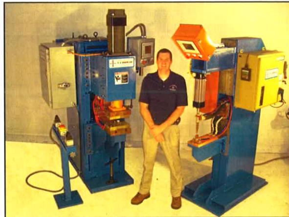
Servo-actuated weld force delivery systems are now being adapted to conventional resistance welding machines, including the press-type projection welding machine on the left and the pedestal-type spot welding machine on the right. Advantages include increased welding speeds and improved process quality monitoring.
