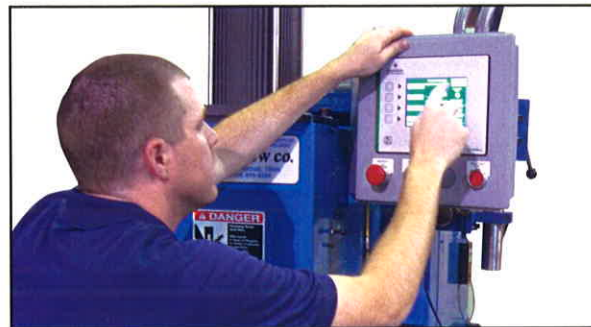
The addition of a touch screen makes a servo-actuated resistance welding machine much more user-friendly.
