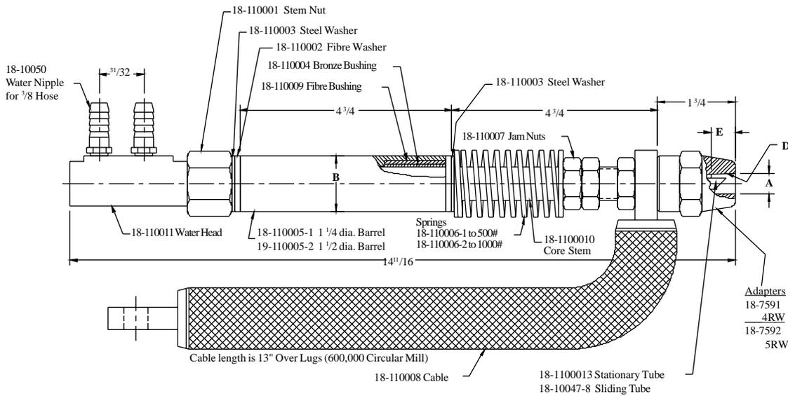
Like other low-inertia holders the heavy duty Adjust-A-Pressure Holders are used for multiple spot and projection welding, and are excellent for indirect welding when mounted in the Adjust-A-Angle Adapter.
