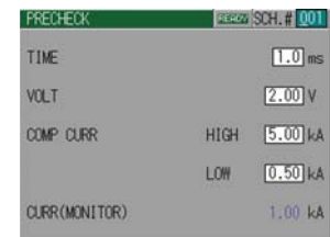
Pre-Check of resistance prior to welding
