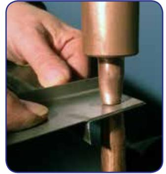
**THE PROBLEM:** Welding their parts required that the operators' fingers had to be close to the moving electrodes. Because of the part design and large number of different models being welded, there was no way they could use drop-in fixtures and anti-tiedown hand buttons.
