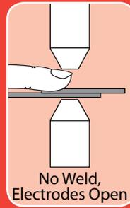
3. If metal is **not** detected, the electrodes open automatically and do not go to welding force. A display tells the operator the problem.
