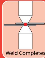
4. If metal **is** detected, full welding force is applied and the weld proceeds normally
