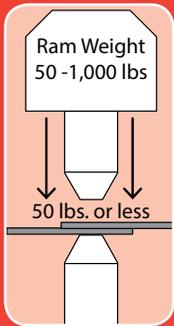
1. The welding electrodes close under **low force**. The unique pneumatic systems designed by UNITROL for this process can counter-balance the weight of the ram on large press welders. Even where the dead-weight of the welder ram is hundreds of pounds, the electrode force produced will be 50 pounds or less.
