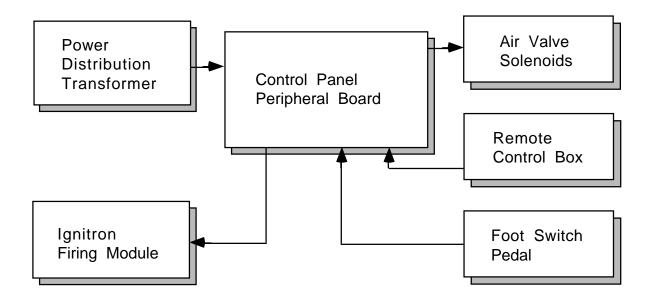
The ignitron firing module package recommended is the model 402B. They should be located in the proximity of the ignitrons whenever possible.
