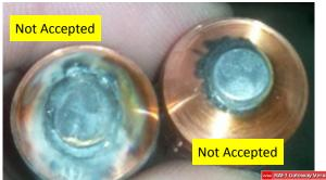
The WTC control can measure precise resistances of welding tips after they have been dressed. Although dressers can remove slag from the edges, the control will identify if the surface of the electrodes are brought back to an approved condition.
