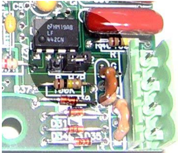
Figure 8-1. Jumper setting: Primary Current Transformer (two pins on the right)
