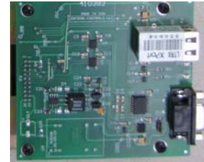
MBTCP/RTU Communication Card P/N 730014-007
