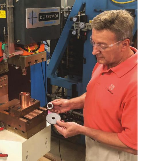
Far left: The use of multiple projections on this curved part allowed the welds to be performed simultaneously. Left: T. J. Snow Welding Engineer Jeff Morgan shows an example of ring projection performed on a part processed on a 20 kJ capacitor discharge welding machine.
