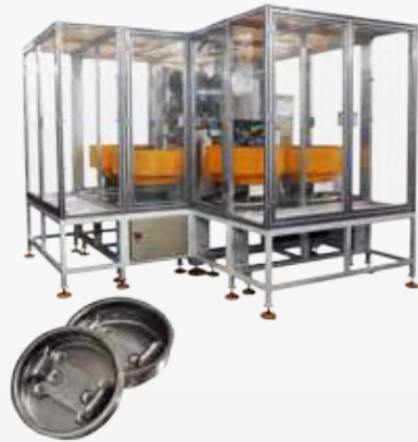
Customized AC Welder For Lamp Holder
