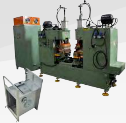
50000J CD Welder For Right Hinge
