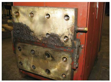
After many years of use, an RW machine's secondary connections can arc and lose conductivity. It is important to re-machine these secondary connections during the welder remanufacturing process. Also, installing a new programmable-type control is recommended as part of remanufacturing a heavy-duty resistance welder from the last century.
