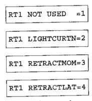
To select LATCHING switch action mode, press 4.
