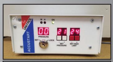
Proper tip force is very important in the formation of a resistance weld. Accustart easily connects to the pressure switch input terminals on any brand resistance welding control.
