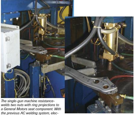
trodes were only good for about 40,000 welds; the new MFDC system enables the machine to run 200,000 welds prior to an electrode change (although just to be conservative, operators change electrodes after 150,000 welds). Annual expenditures for consumables has dropped by more than \$10,700.
